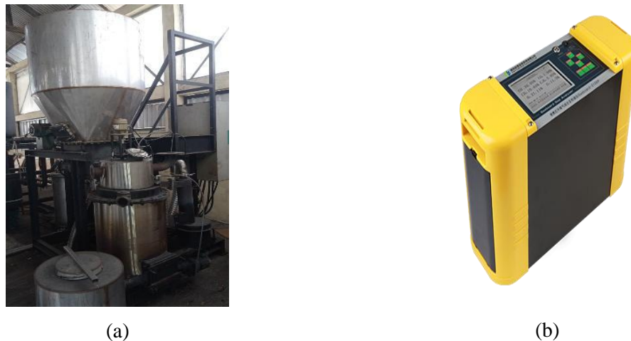
Fig. 1. Tools used in this study: 15 kWh downdraft gasifier reactor (a) and portable infrared syngas analyzer gasboard G3100-P (b).
